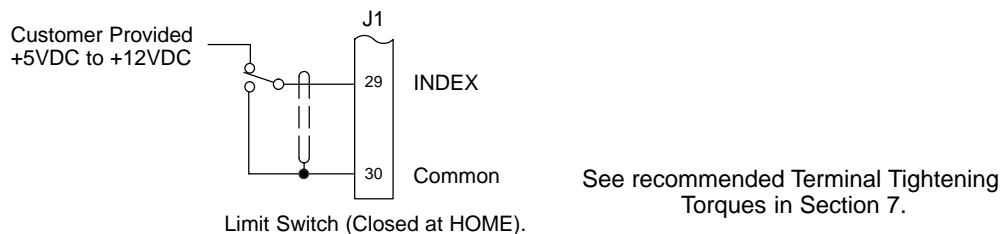
Figure 3-26 Typical Home or Orient Switch Connections
