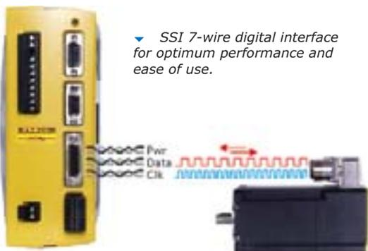
▼ SSI 7-wire digital interface for optimum performance and ease of use.
